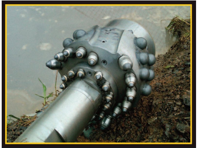
Completed 570 feet of solid shale finished backream, May 2013
