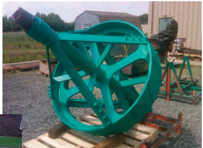
Completed 570 feet of solid shale finished backream, May 2013
